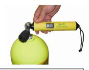
Use Independent Oxygen Analyzer for Verification
